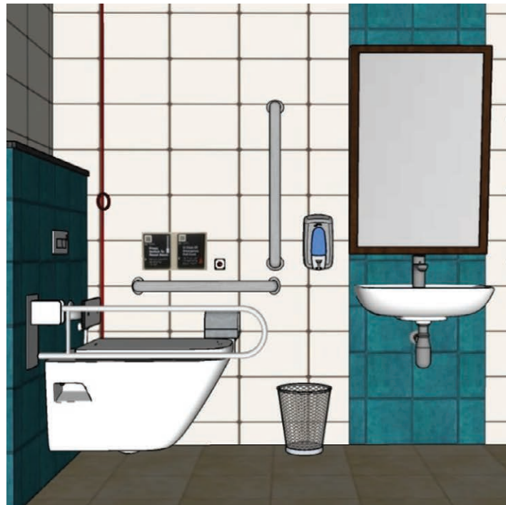
Figure 18 Gender neutral accessible toilet
