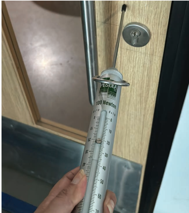
Figure 6 Measuring door opening force during an access audit
