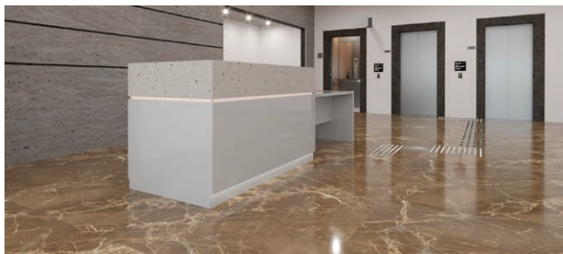
Figure 14 Accessible Reception Counter
