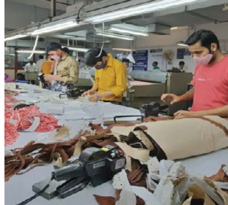
Ticketing of cut garment – Repetitive work; requires checking / adjusting unique number on the ticketing machine (accessible interface missing), good hand dexterity must
