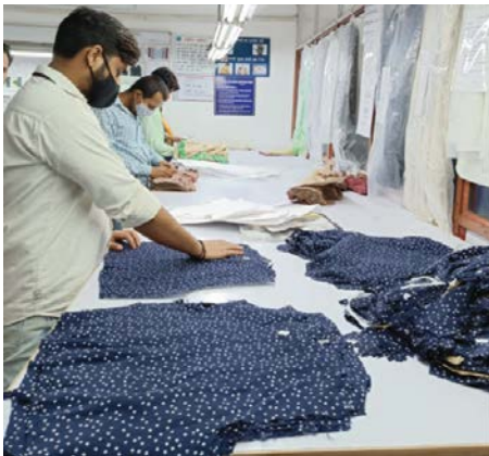
Bundling of cut garments – Repetitive work; requires standing for hours, layering cloth (seem by seem), bundling and numbering as per ticketing sequence
